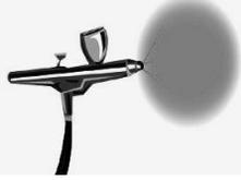
Apply in light coats. A coating consisting of multiple, light layers is much stronger than a coating of the same mil thickness which is achieved in fewer, thicker layers. Chipping and flaking of paint is most often due to excess build-up of paint. Allow colors to air cure between coats and before curing with heat (see curing section for more). Working in light coats is especially important when painting flexible surfaces such as leather and vinyl.
