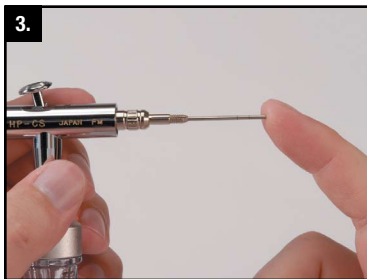
3. GENTLY push on the back of the needle to make sure it is seated into the nozzle. (image 3)
