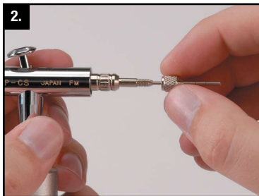
2. Remove needle chucking nut. (image 2)
